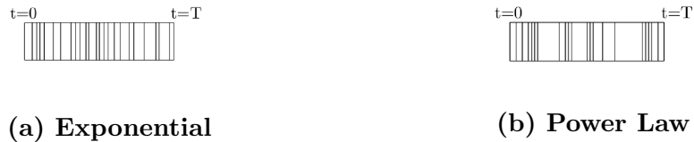
Figure 2.3: Comparison between interaction streams with (a) exponential wait times and (b) power law wait times. The power law wait times result in bunches of interactions mixed with longer periods of down time.
