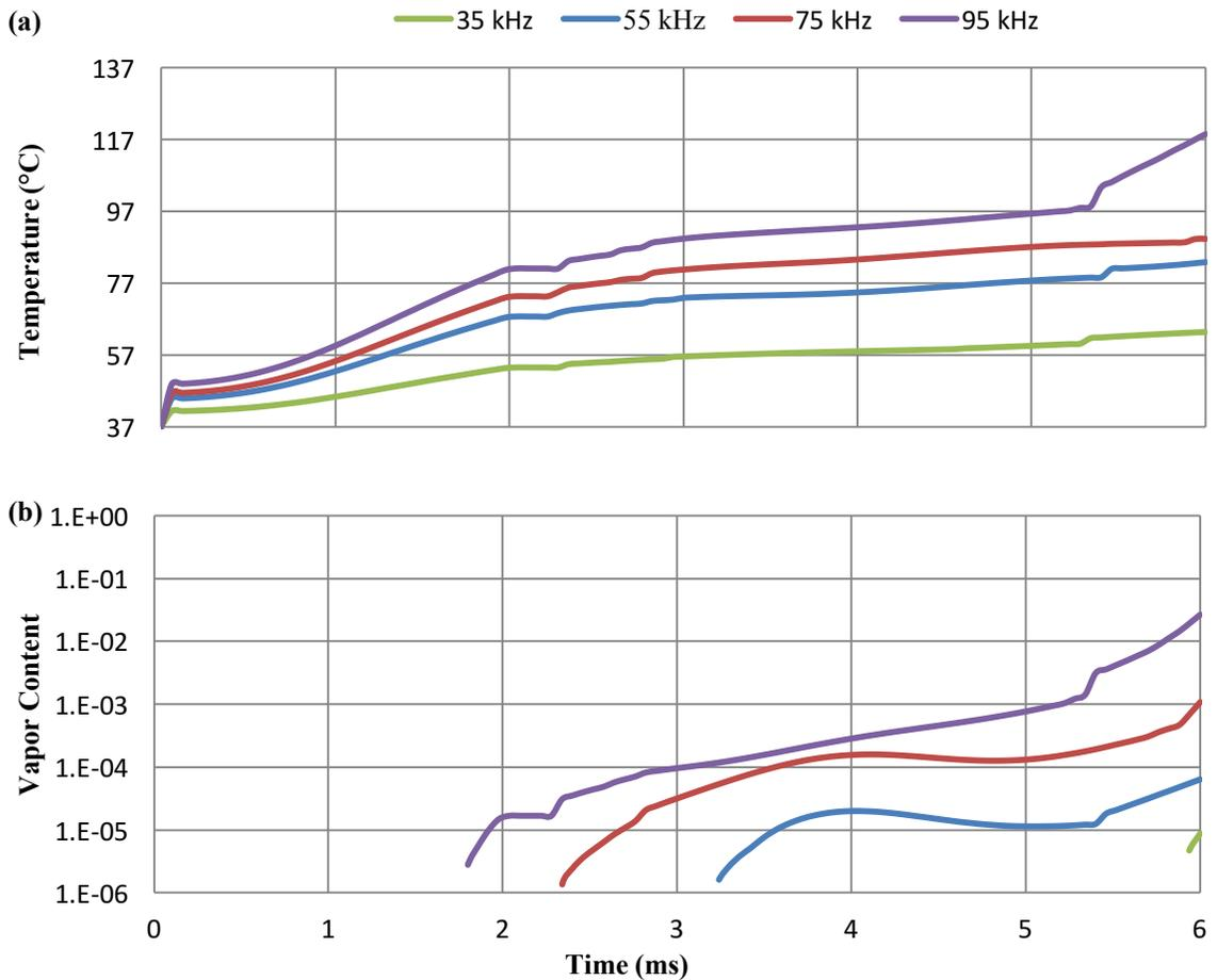
Figure 11. Evolution of temperature and vapor content with different frequencies. (a) Temperature vs. time with different frequencies. (b) Vapor content vs. time with different frequencies.
