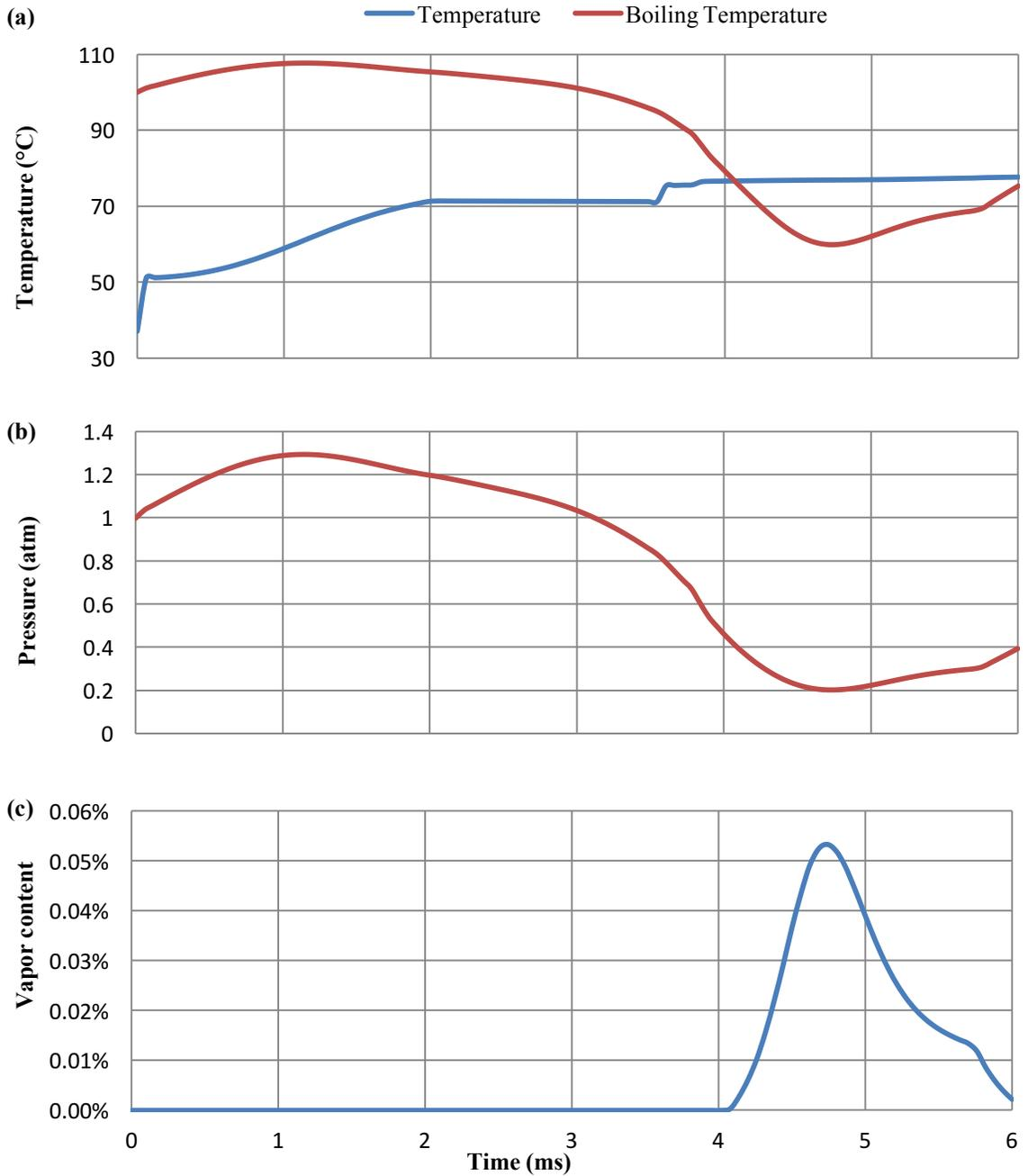
**Figure 10. Evolution of temperature, pressure and vapor content. (a) Temperature and boiling temperature vs. time. (b) Pressure vs. time. (c) Vapor content vs. time.**
