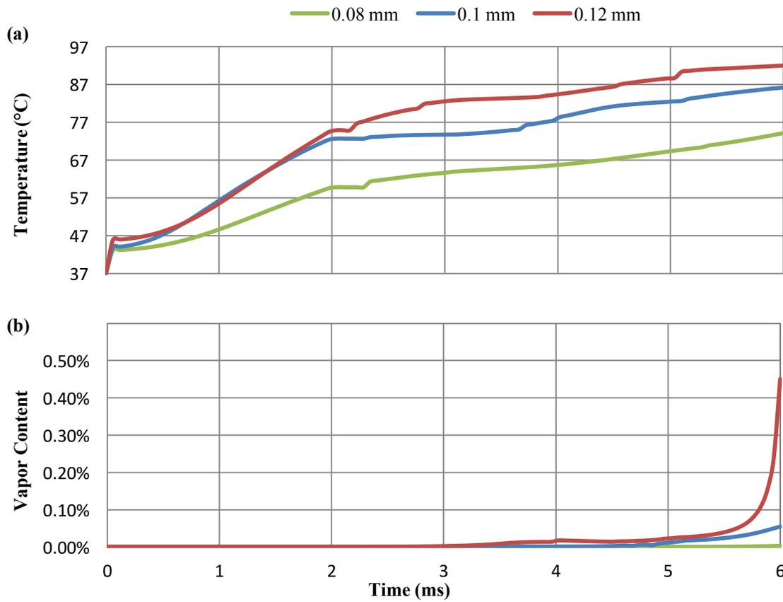
Figure 12. Evolution of temperature and vapor content with different loadings. (a) Temperature vs. time. (b) Vapor content vs. time.
