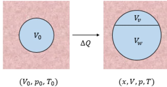
**Figure 1. Demonstration of the cavitation model. Heat is added to a spherical cavity initially filled with water surrounded by an infinite elastic medium, resulting in a fraction of water ( $x$ ) converted to vapor and changes in volume, pressure and temperature.**
