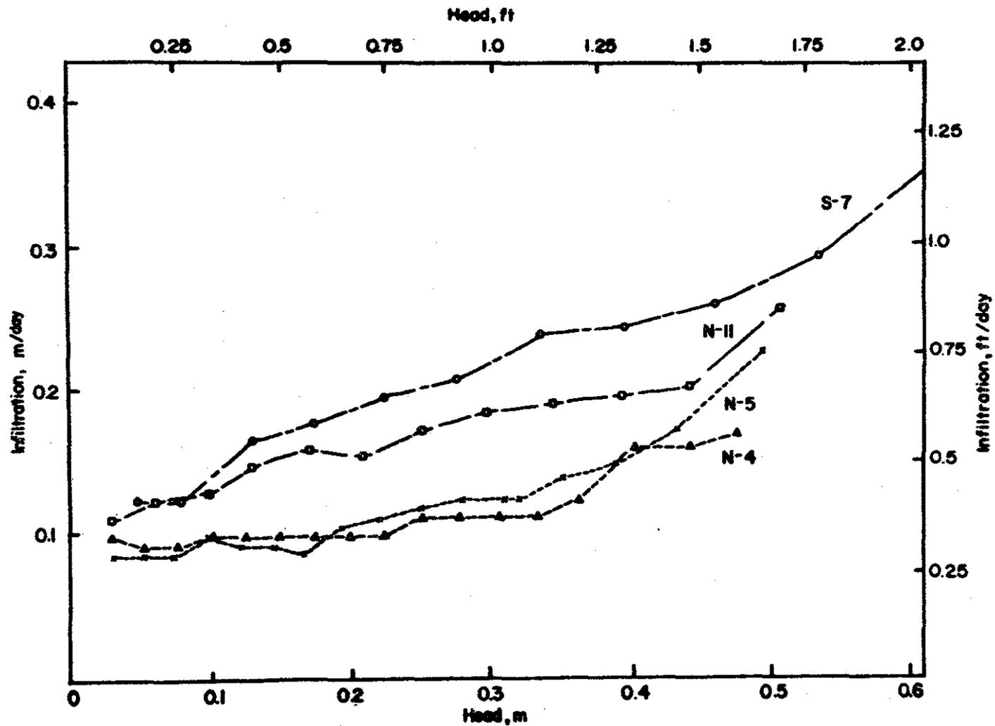
FIG 3.- Infiltration Rates of Several Sand Beds in Normal Use
