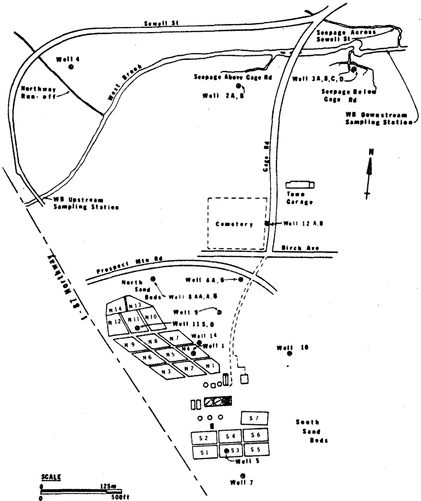
FIG 4.- Area of Study Showing the Treatment Plant, Observation Wells, and Seepage into West Brook
