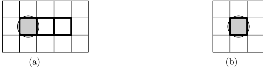
Figure 3.5: The sizes of a mixer and a storage unit. (a) A mixer with 3 electrodes for droplets to move. S_{mix} = 15 . (b) A storage unit with 1 electrode for droplets to stay. S_{store} = 9 .
