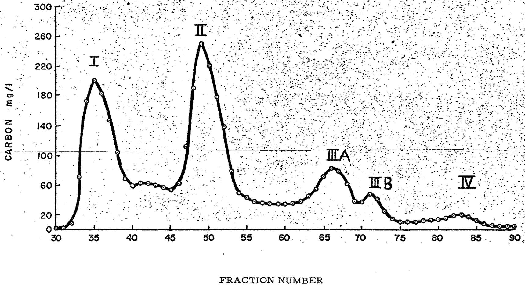
Figure 1. Fractionation of Batavia (1-22-69) Concentrate on Sephadex G-10. Sample Volume: 10 ml, Bed Dimensions: 2.5x85 cm, Flow Rate: 50 ml/hr, Eluant: Glass Distilled Water.
