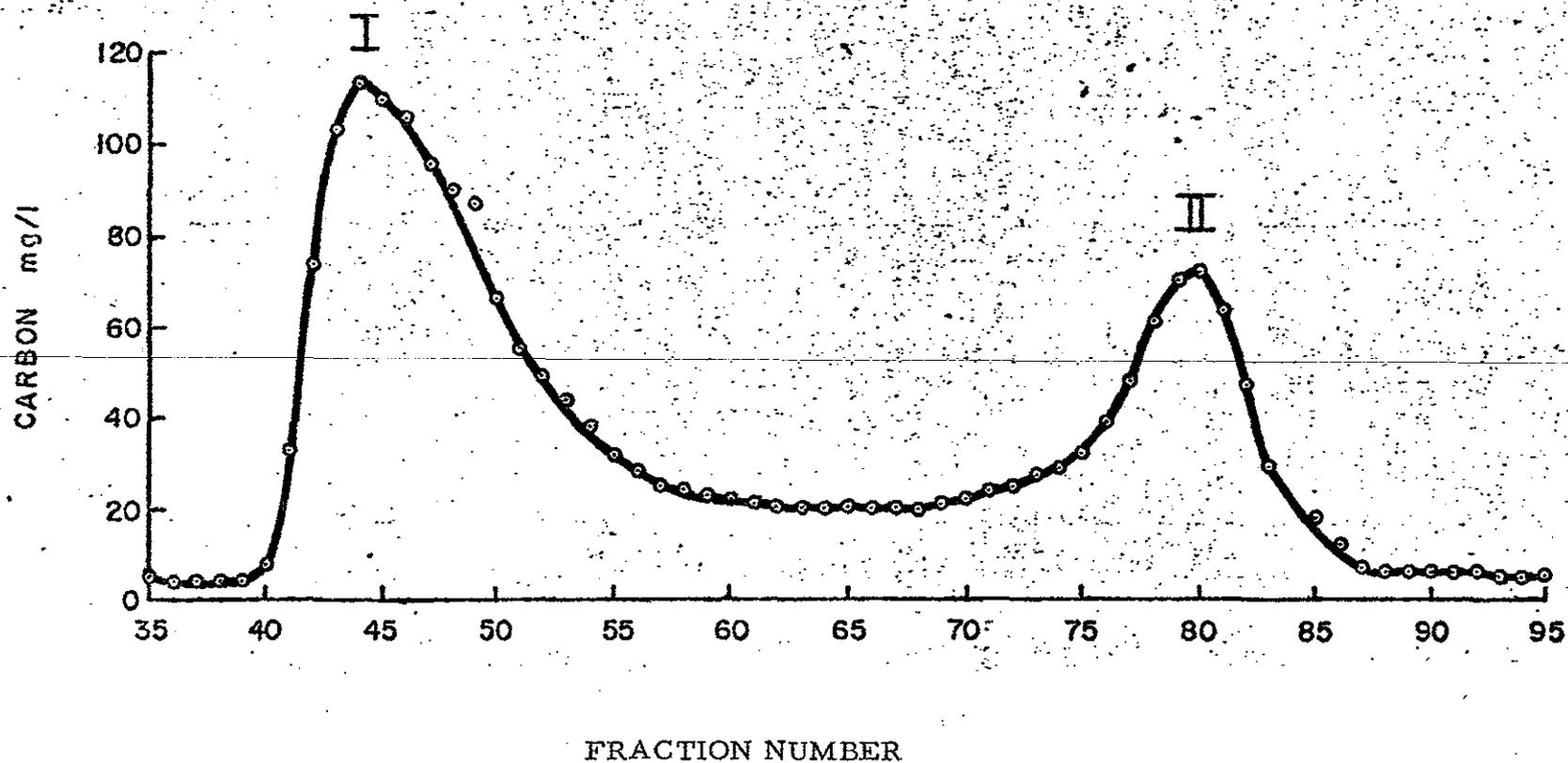
Figure 2. Fractionation of Composite Fraction G-10-I on Sephadex G-25. Sample Volume: 10 ml, Bed Dimensions: 2.5x90 cm, Flow Rate: 135 ml/hr, Eluant: Glass Distilled Water.
