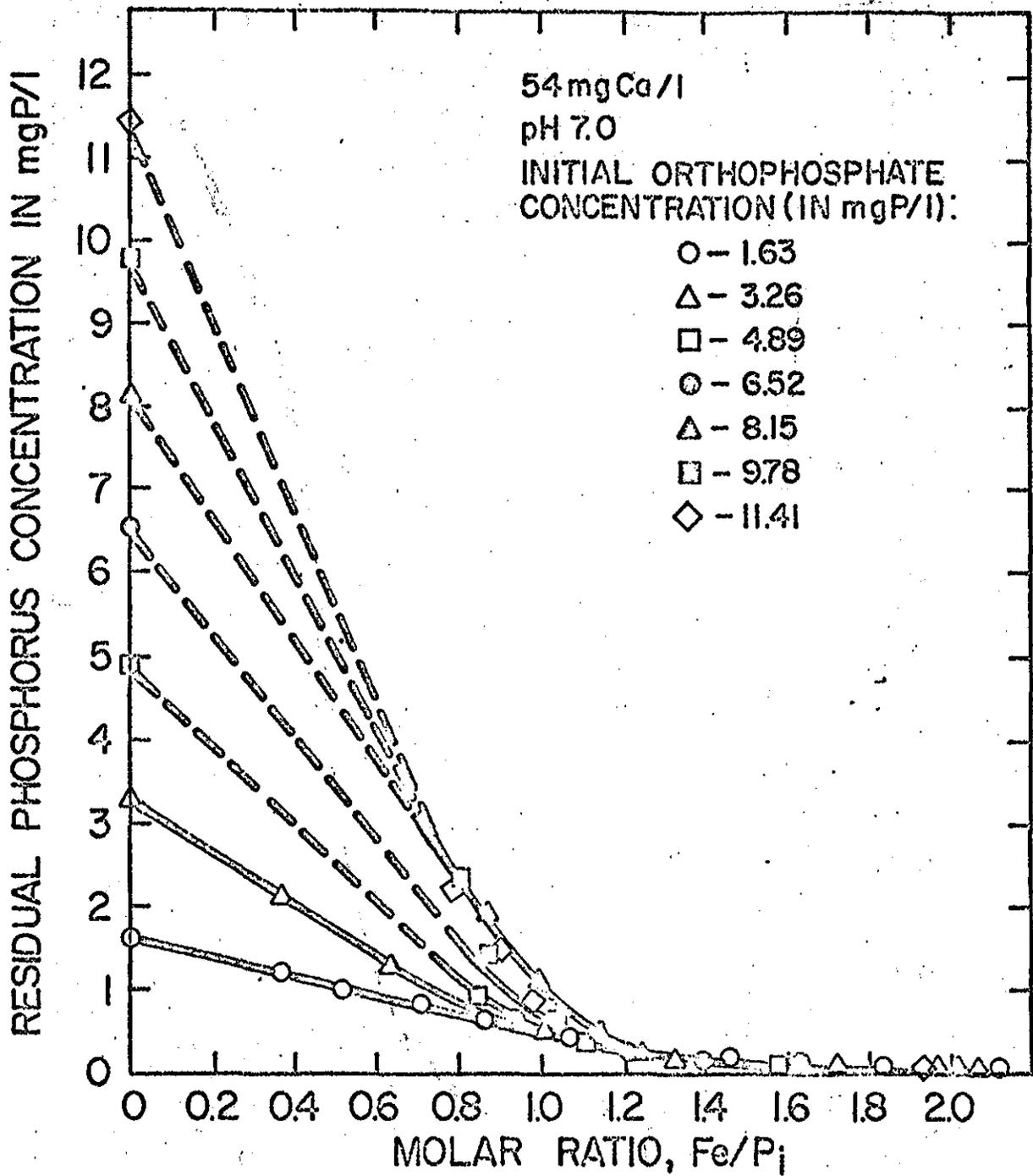
FIGURE 3. THE EFFECT OF COAGULANT CONCENTRATION (MOLAR RATIO, Fe/P<sub>i</sub>) ON THE CONCENTRATION OF RESIDUAL PHOSPHORUS
