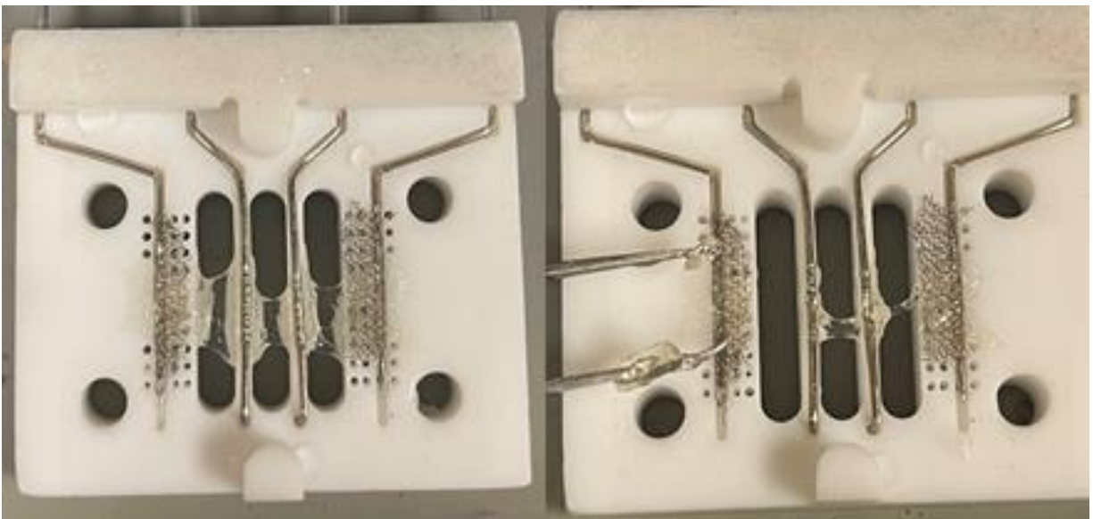
Figure 31. PS(QA)-2.02 after OH - conductivity measurement at 80°C, the film does not maintain its form, is very gel like, and is impossible to collect in one piece.
