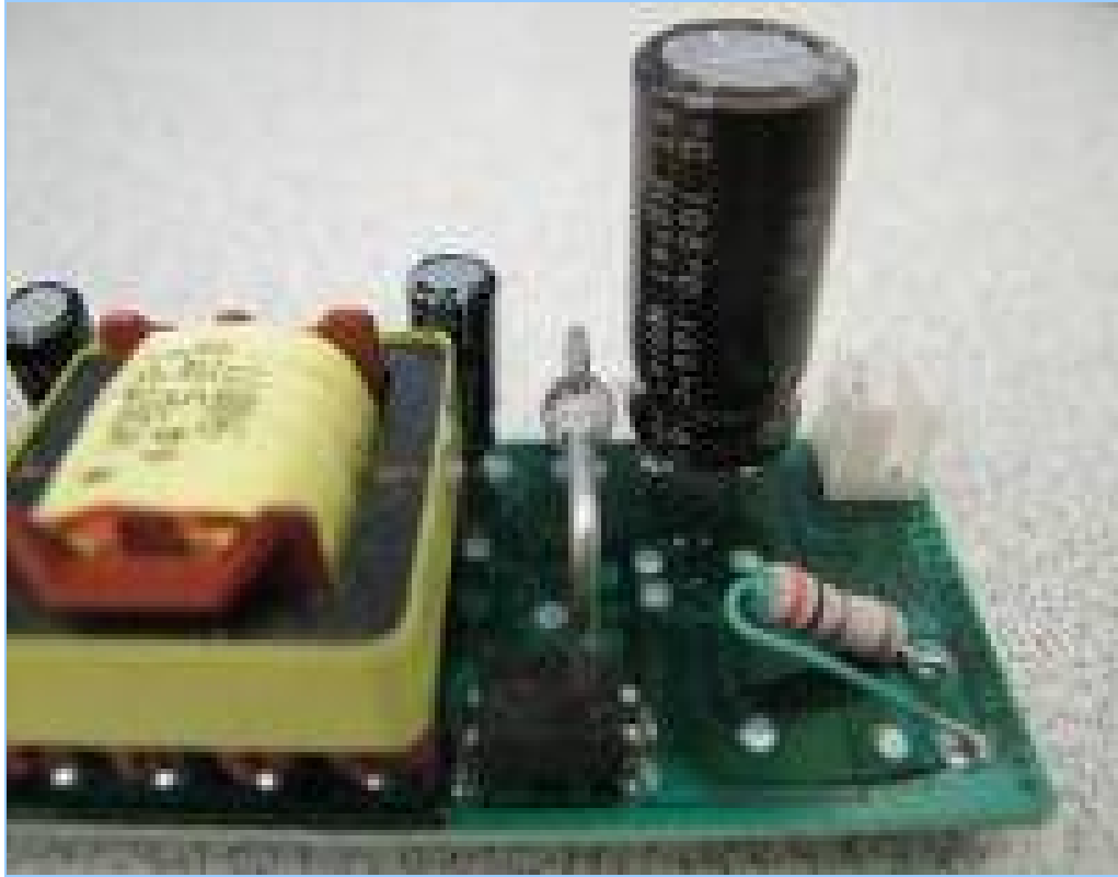
Fig 3-3 An electrolytic capacitor at output stage of LED driver B
