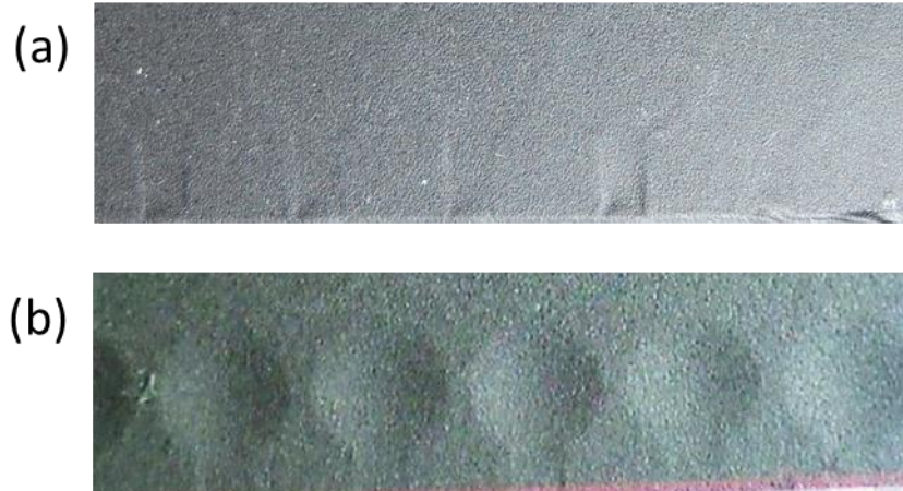
Figure 2. EAP actuator (a) before and (b) after an external voltage difference is applied.
