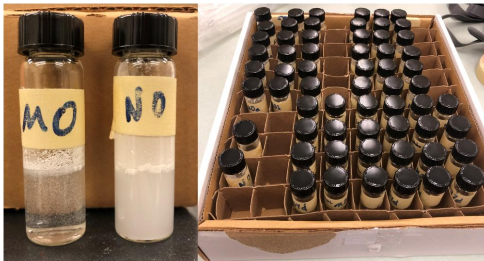
Figure 5-5. Vials of creatinine solution containing MIP (“M0”) and NIP (“N0”). Left photo taken after agitating the solution.
