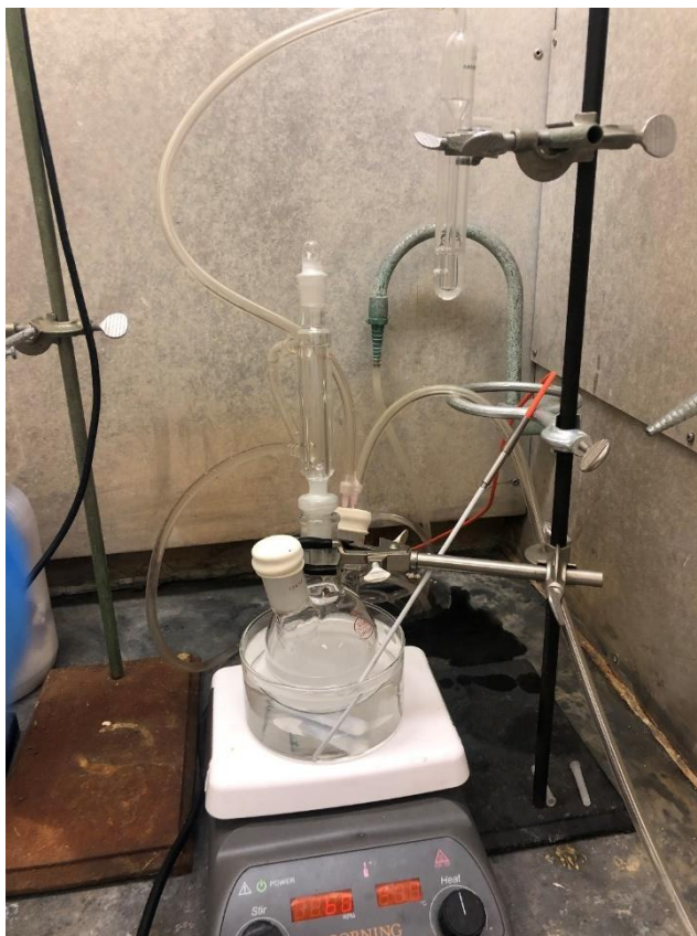
Figure 4-3. MIP synthesis apparatus photograph.
