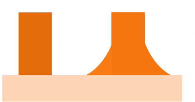
Figure 31: Traces with orthogonal walls provide more predictable electrical behavior than traces with incomplete etch profiles.
