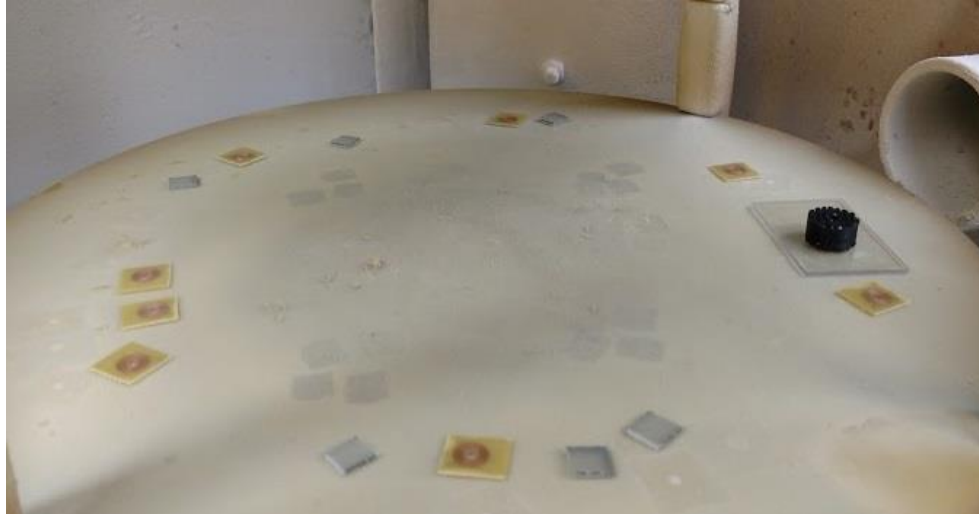
Figure 37: Coils were placed roughly at the same radius from the center of the platform for consistent deposition for each batch.
