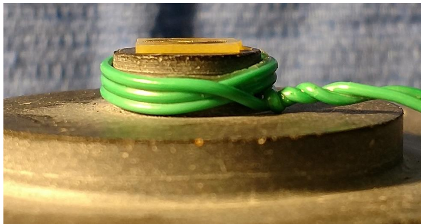
Figure 49: The machined AlSi fixture allows for continuous monitoring of coils and sensors during testing.
