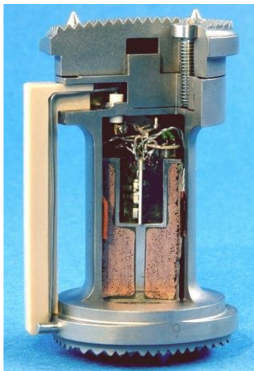
Figure 7: Rohlmann et al 's smart anterior vertebral replacement was used to measure in vivo forces in the lumbar spine [42].
