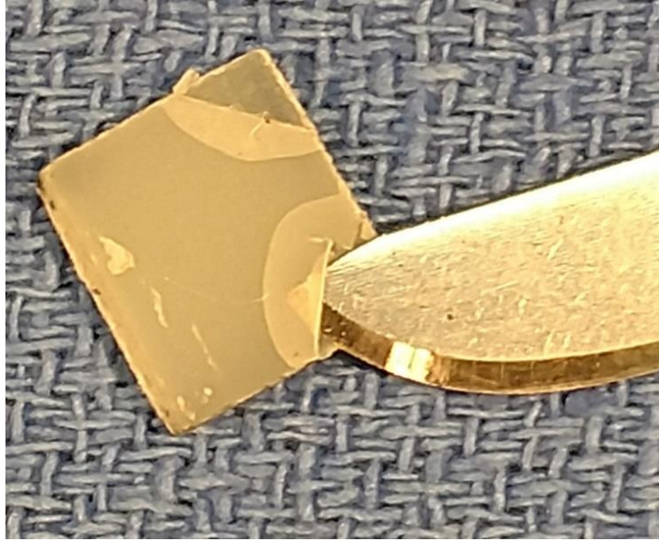
Figure 32: Untreated substrates coated with parylene C easily delaminates when a sharp edge is inserted between the substrate and parylene C. The lighter colors near the corners indicate delaminated parylene C.
