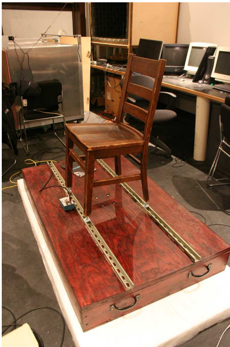
Figure 5.5: Motion platform used in multimodal presentation of audio-tactile stimuli. Sennheiser HD280 headphones are used for audio presentation.
