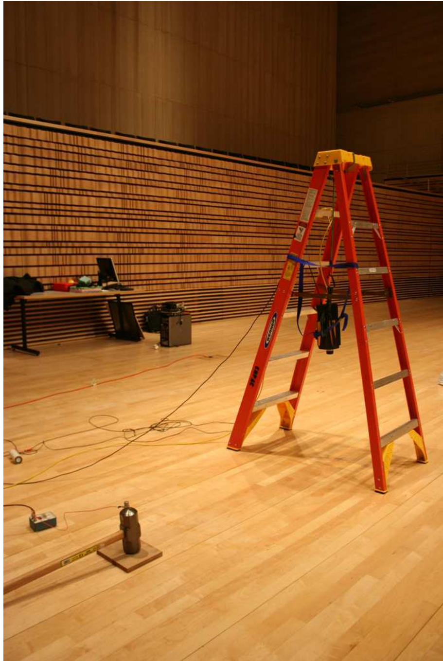
Figure 5.4: Structural impulse response measurement equipment. Instrumented sledhammer used to measure force input, laser doppler vibrometer used to measure force output (isolated from stage with bungee cord). Not Shown: 150 lbs of sand placed on chair used to mass load receiver position, source position mass loaded by experimenter operating hammer.
